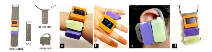
Diafit includes accessories and feedback modules for building different styles of glucose monitors such as: (a) bracelet monitor, (b) ring monitor, (c) earpiece monitor and (d) necklace monitor.
