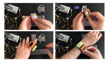
Using modular design as the basis, DiaFit allows people to assemble different combinations of glucose monitors using accessories (e.g., monitor as a bracelet) and feedback modules (e.g., change in glucose level to be felt via vibration and visual display).
