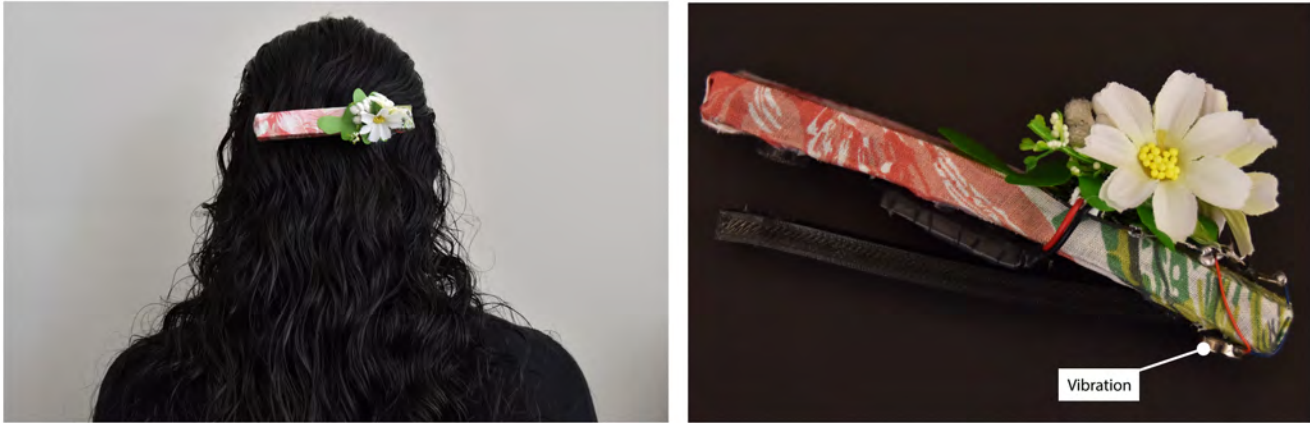
Figure 14: The developed hairclip-based monitor worn by a user on the left, and showcasing its embedded circuitry on the right.
