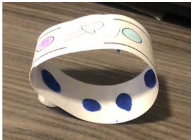
(a) A ring with vibration (represented by Play-doh on the inner band) as its primary alerting mechanism.
