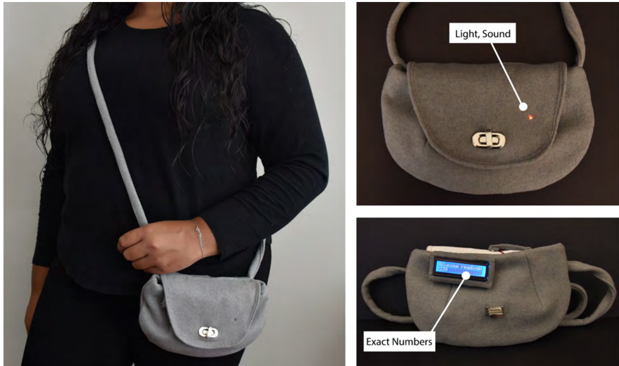
Figure 13: The developed purse-based monitor worn by a user on the left, and the provided feedback on the right.
