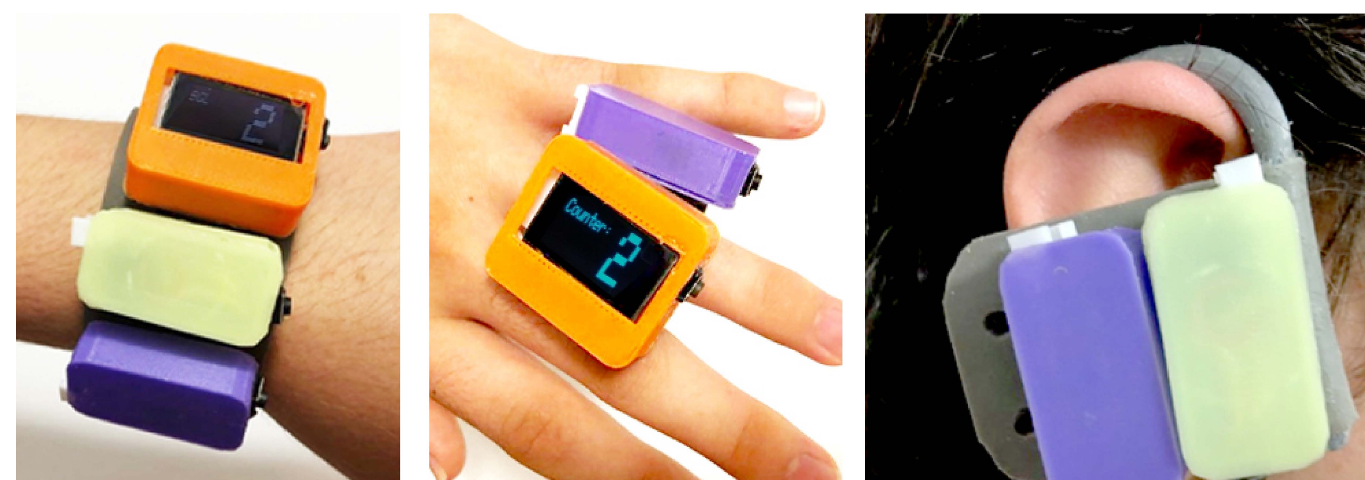
Figure 2: Examples of do-it-yourself (DIY) 3D-printed glucose monitors [2].
